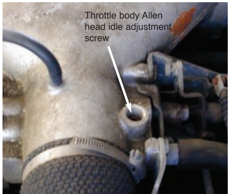
Figure 3. Location of throttle body allen screw adjustment screw, shown with tamper proof plug # RNM109 removed.
