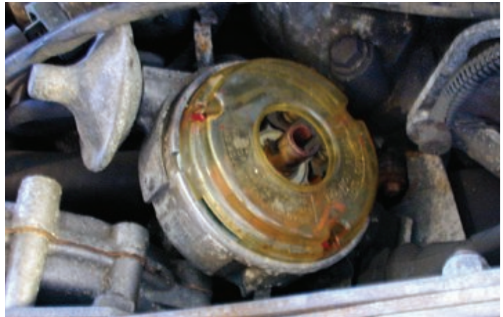
Figure 1. Dust cover screws are marked with red paint - don't loose them!
