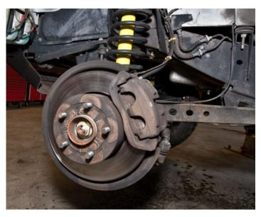
Step 3. For the majority of owners, the rotor hat and a few other bolts will be rusty. Ideally if you have the time, spraying PB blaster on all the bolts you plan on removing and letting it sit for a while would be ideal. I sprayed all the bolts and let it sit for about 20 minutes.
