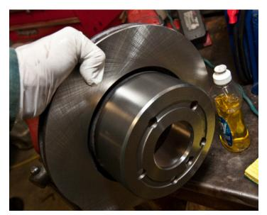
**Step 10.** At this point it is ideal to wash all of your rotors with either brake cleaner or dish soap and water. Make sure to clean it thoroughly to get rid of any soap or grease on the rotor.
