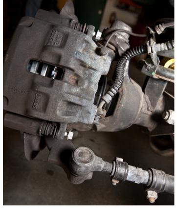
Step 13. Now complete the steps in reverse. Unscrew the brake fluid reservoir before compressing the pistons. You'll need a piston compressor, or some sort of clamp that can compress the pistons on the caliper(2) so you can slide the caliper over the pads on the rotors. after doing that, located on of the bolts on the caliper, and screw it halfway. Then insert the other caliper 12mm bolt, once located, torque both to \_\_\_
