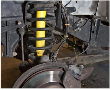
Step 5. It is important at this point to support the caliper itself. You do not want any stress on the brake line, it could cause damage and leave you in the shop for a lot longer. I used a coat hanger, but bungee cords are ideal for this.
