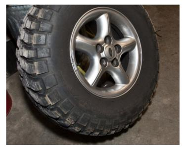
Step 2. Remove the rest of the lug nuts and remove the front wheels. I want to stress that this job does not require a large amount of tools and special skills, it is quite easy and can be done with a small selection of tools.
