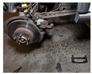
**Step 7.** Now that you have removed the bolts and caliper mount, you have access to the rotor. At this point, you'll have wanted to have sprayed the rotor mounting screw a few hours ago.
