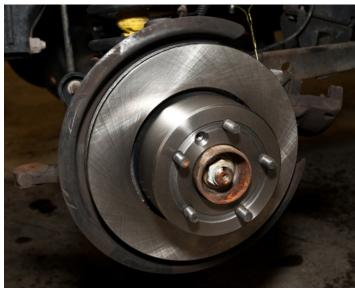
Step 12. After cleaned up, slide the rotor onto the wheel studs. It should be a tight fit so that it remains snug. Install caliper hangers over new rotors, torque 19mm, 12-point bolts to\_\_\_\_.
