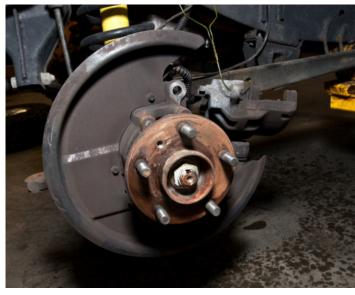
Step 9. Now that you have removed the rotor locating screw, and slid off the rotor by hand or with a rubber mallet, this is what you'll be looking at. It is important that when handling the new rotors you use gloves to make sure you don't get oil or grease on the new rotors.
