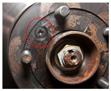
**Step 8.** Welcome to your worst nightmare. This little devil is the rotor locating screw, and it is the bane of my existence. For some reason, the one on my rotor hat was already stripped, so I didn't get it easy. The way I finally completed the removal, was by torching the screw and hammering a flathead into it. You may get lucky and get it out with a screwdriver, but I severely doubt it. Good luck with this step, it is painful.
