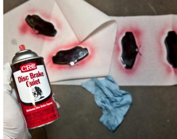
**Step 11.** Spraying your pads with anti-squeal spray or copper anti-seize paste is a good idea at any point of the install. Anti-squeal will have to dry, so it might be best to clean around the hub while it is drying.
