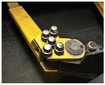
Step 1. Using a lift to do a brake job is quite ideal, although it can be done without one using jacks and jackstands. You'll want to break tension on the lug nuts before raising the truck in the air. Use a wrench instead of an impact drill to prevent damage to the lug nuts.
