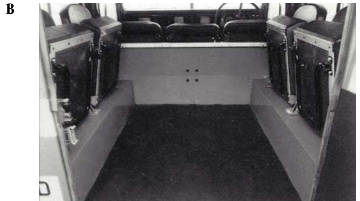
Correct location of seat base when folded up
