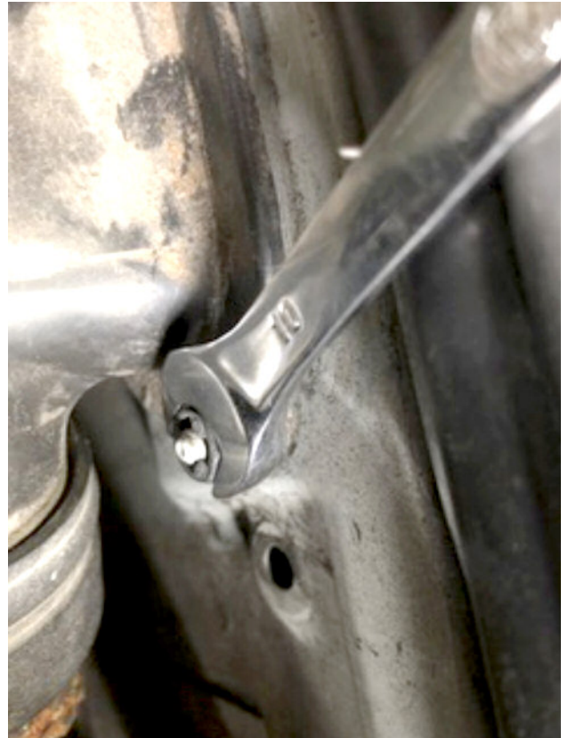
Step 2. Using the 10mm wrench undo the two plastic nuts on each side at fender junction.
