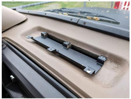
When installing the top piece, you may have trouble reaching the back tabs with the provided screws. In this case, you can temporarily use a longer M4 screw to "catch" the tab and bend it upwards.
