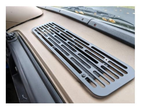
When installed correctly, the grid should fit nicely in the recess and sit flush with the rest of the dashboard. It should feel very solid.
