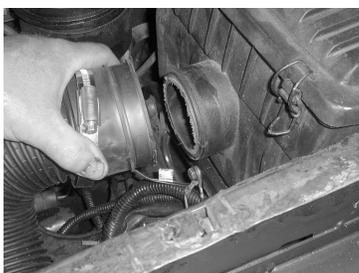
Saw off the end of the air trumpet as shown above and, using the supplied clamp, attach the new flexible air intake hose directly to the air filter box. Note that you may need to relocate the jack and wheel chuck if necessary to allow the tube to attach to your air filter box.
