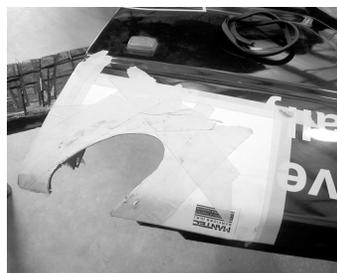
Use MANTEC's template as shown to cut the fender hole. Be sure to thoroughly tape off the template to protect the paint around the hole. Make sure to first cut conservatively inside the trim line and fit several times until the fender is snug to the pipe with room for the gasket.
