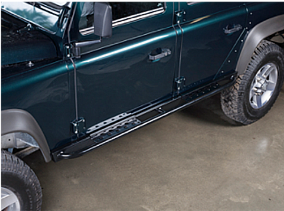
Figure 7: An example of the rock sliders properly installed, paired with optional black modular tread plates (RNA1080SS).
