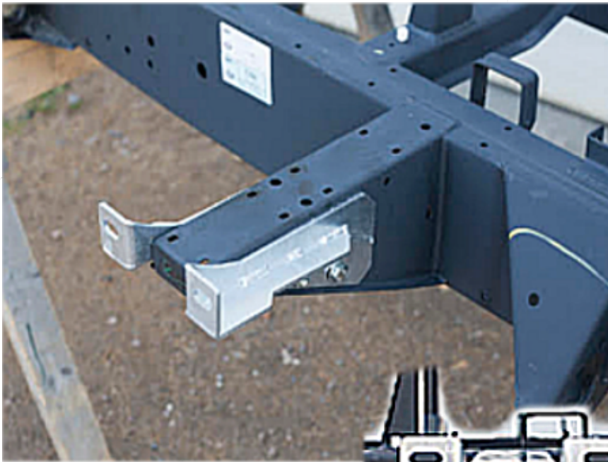
Figure 3: Middle brackets, properly mounted.
