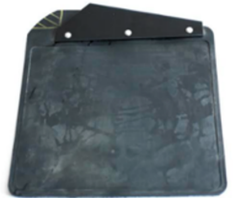
Figure 8: To reinstall mudflaps a small cutout, such as the one drawn above, will be necessary.
