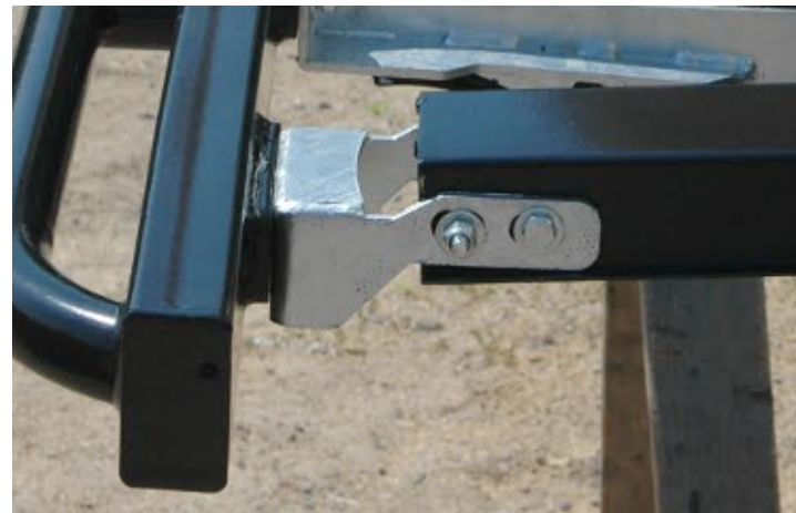
Figure 4: Rear bracket, fitted to middle floor crossmember.
