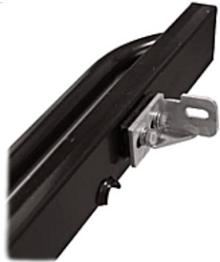
Figure 2: Forward bracket, properly mounted on rock slider.
