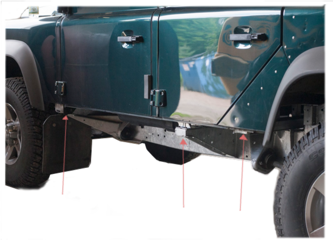
Figure 1: Sills removed, chassis mounting points exposed.
