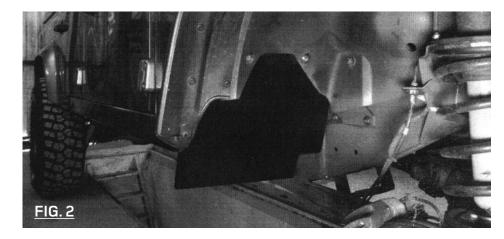
4. To the right shows how to orientate the shields when looking from the front of the vehicle. Note the cut out for the radius arms (Figure 3).
