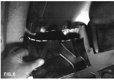
Figure 6 at left shows the part of the inner arch you need to remove, once removed you can slide our Mud Shield up in place as per the main instructions above.
