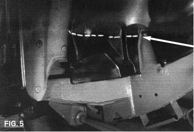
The easiest way to cut this inner arch is to follow the dashed line as in the Figure 5 to the left. Make sure you cut below the two screw fittings.
