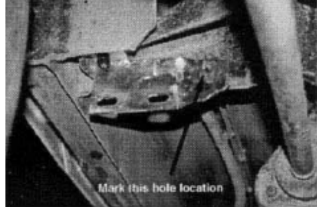
Fig. 6 Detail mark hole location as shown
