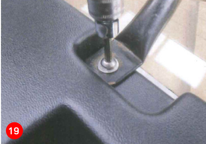
Step 19. Refit the grab handle using the new socket headed bolt provided. Use a 4mm hex Allen Key.
