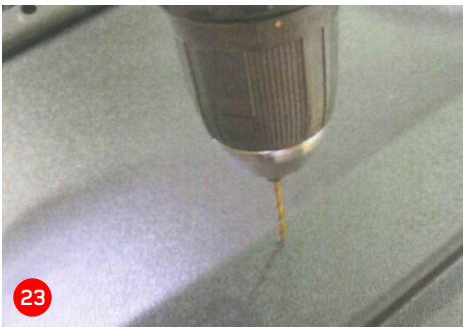
Step 23. Drill through the trim using a 3mm drill bit.
