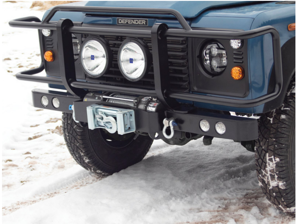
RNA2120 shown above with optional Brush Guard, Winch, Recovery Points, and Hella Rallye 4000 Lights
