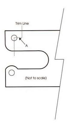
Note: After trimming, an alternate bolt hole will not be necessary, but can be added at the installer's discretion.
