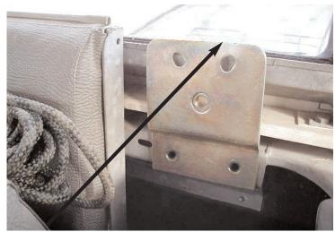
**4)** Illustration of inertia reel assembly mount. Left hand reel is mounted to forward hole shown by arrow
