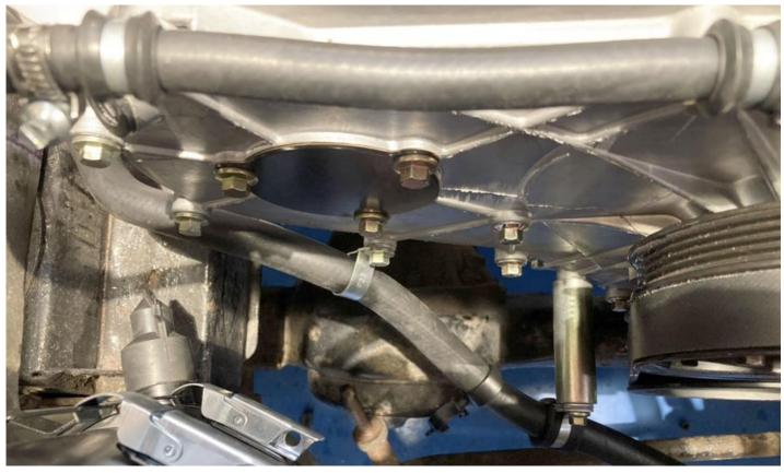
**16.** Cooling hoses: Fit the top hose and extension hose, using the Revotec thermostat as a joiner. Ensure all hose clips are tight. See picture right.
