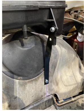
Remove fan cowl plates: these are fixed to the front wings on either side.
