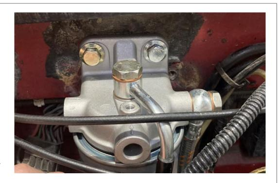
Fit the 226–17–04 fittings with nut and olive to the lift pump inlet and outlet tube.
