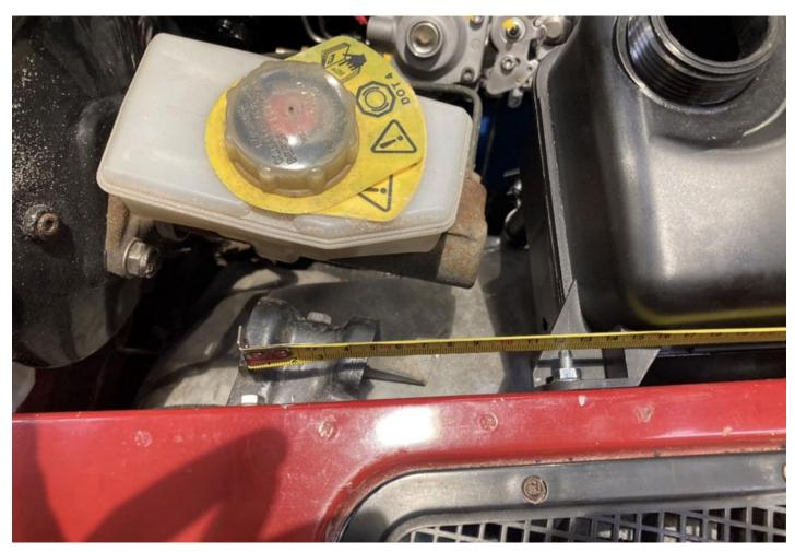
Header tank: Fit the header tank to the wing with appropriate fixings. Then fit the ESR213 bracket to the header tank and use as a jig to locate the bottom hole for the bracket. When the bottom hole location is found, drill another 6.5mm hole into the inner wheel arch; ensure that the bottom hose connection has sufficient clearance from the inner wheel arch. Remove header tank and bracket and ensure all holes are deburred. See picture right.
