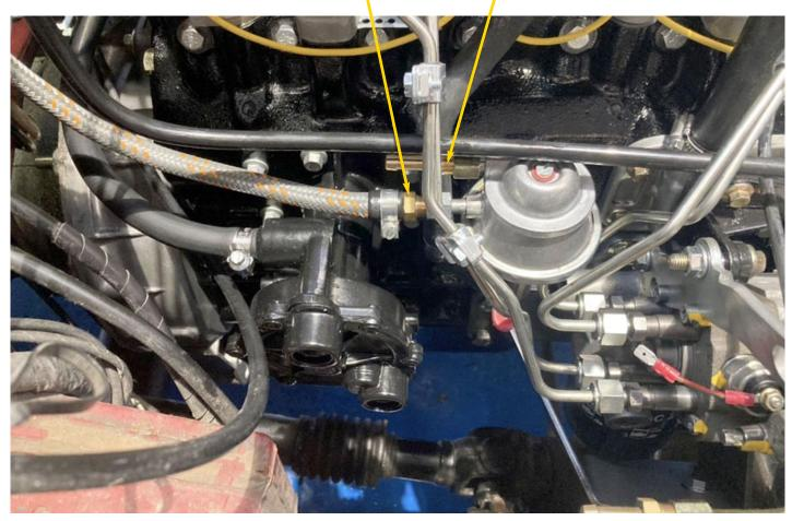
Fitting the New Engine -Fuel filter, pipes
