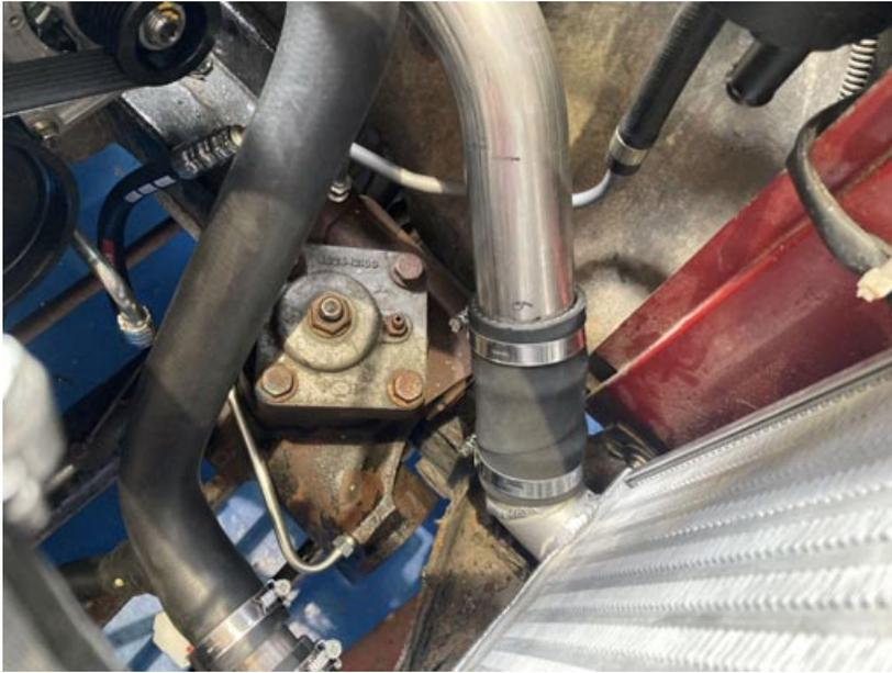
12. Intercooler to inlet manifold hose: Fit the standard LR ESR2309 hose to the intercooler, stainless joiner and hose extension. See picture below.
