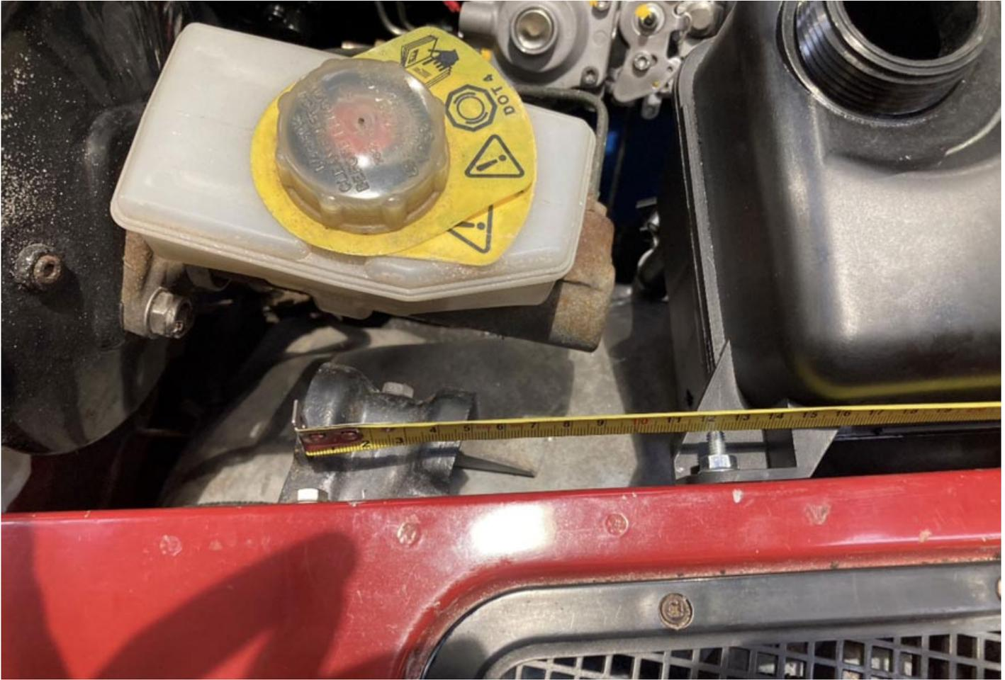
6. **Header tank:** Fit the header tank to the wing with appropriate fixings. Then fit the ESR213 bracket to the header tank and use as a jig to locate the bottom hole for the bracket. When the bottom hole location is found, drill another 6.5mm hole into the inner wheel arch; ensure that the bottom hose connection has sufficient clearance from the inner wheel arch. Remove header tank and bracket and ensure all holes are deburred. See picture right.
