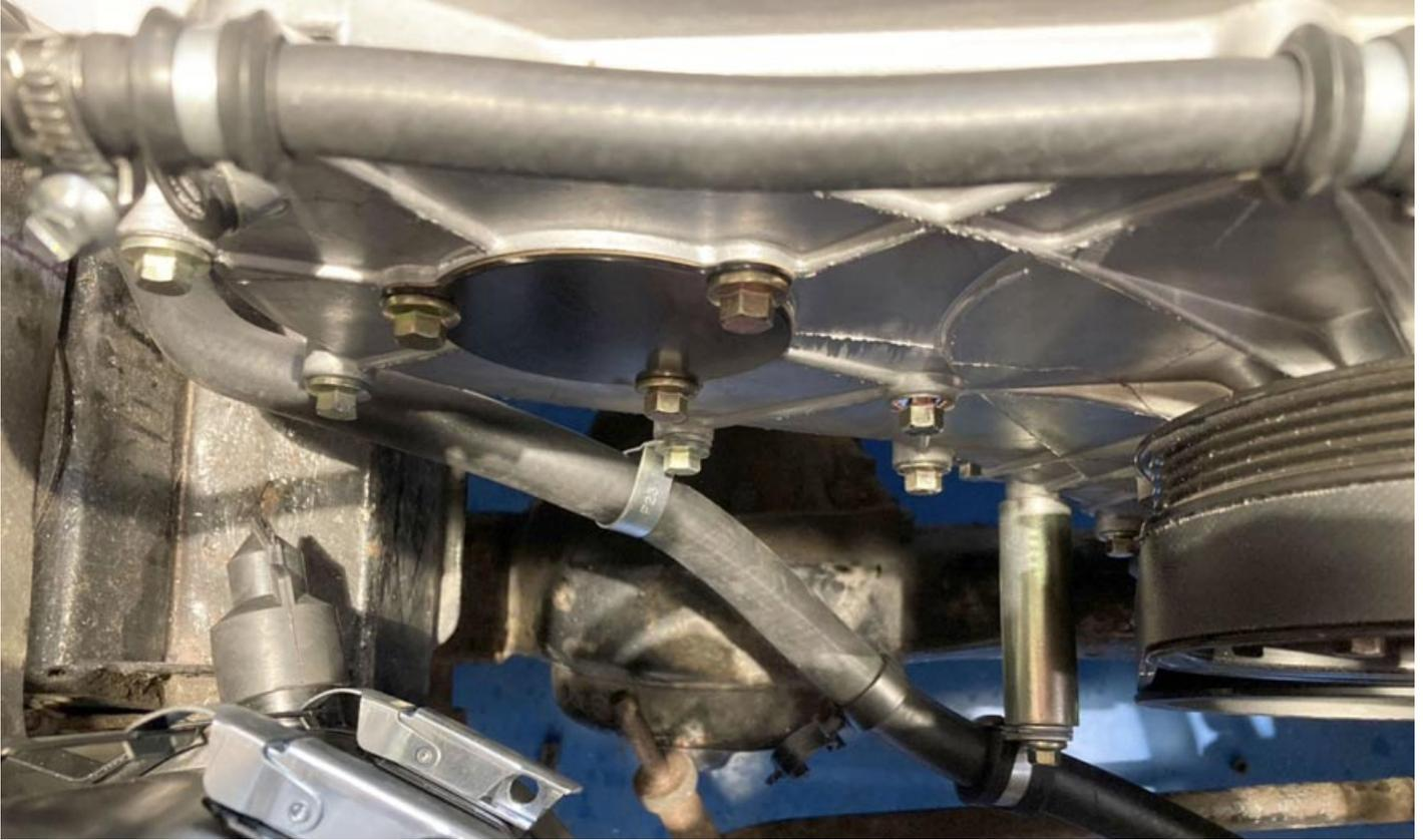
16. **Cooling hoses:** Fit the top hose and extension hose, using the Revotec thermostat as a joiner. Ensure all hose clips are tight. See picture right.
