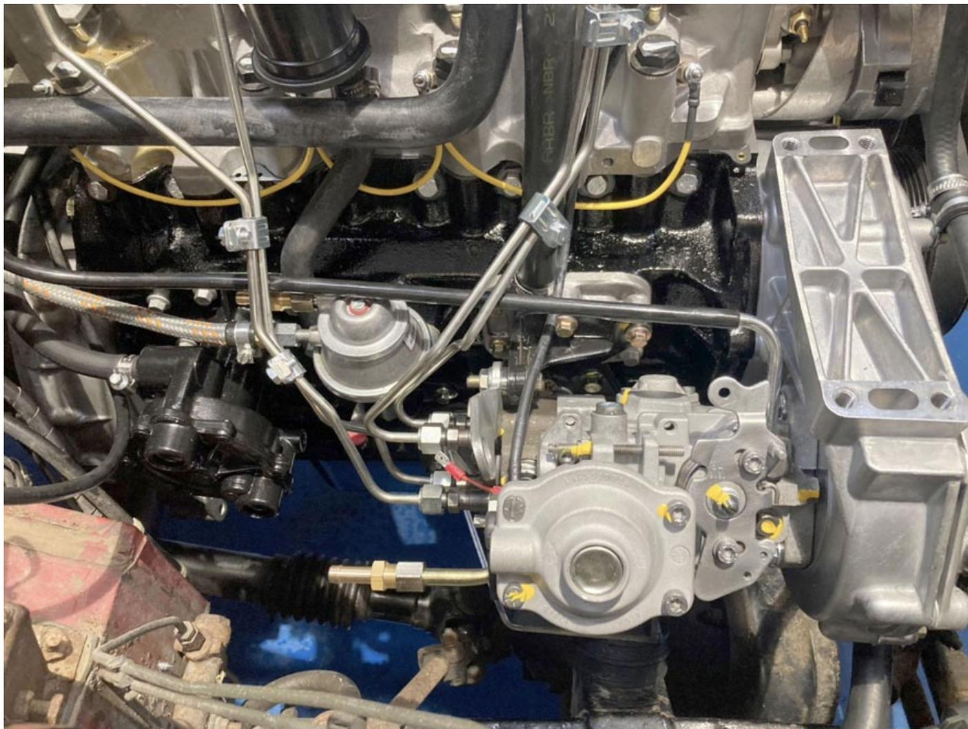
**27. Fuel filter and pipes:** The lift pump inlet and injection pump return now has an 8mm barbed fitting. From the original fuel pipes for the original engine, fit a length of 8mm hose with hose clips to the new fitting for both flow and return.
