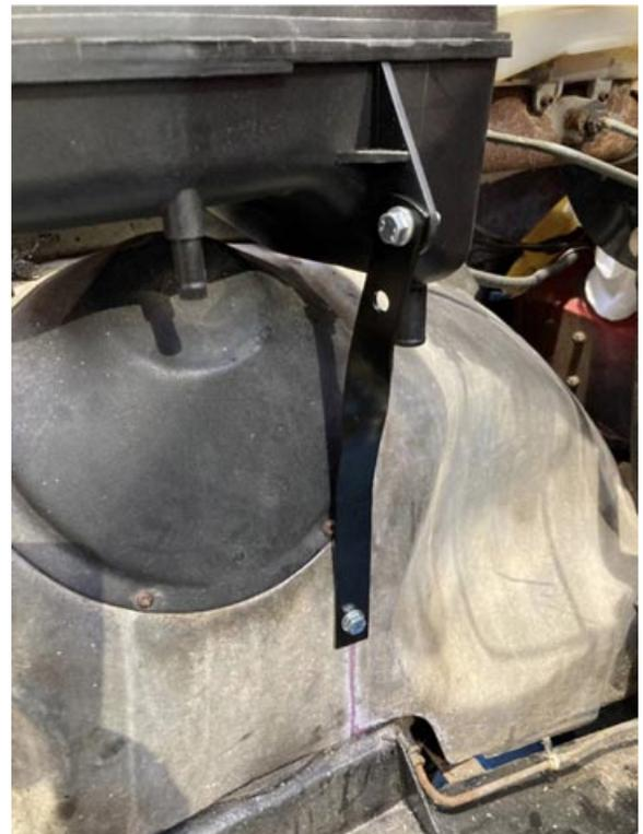
7. Remove fan cowl plates: these are fixed to the front wings on either side. See 2 pictures this page.
