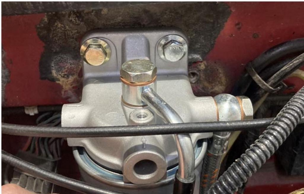
24. Fuel filter and pipes: Fit the 226-17-04 fittings to the lift pump inlet and outlet connections. Nut, then olive, then fitting. Tighten nut to fitting; ensure that the fitting is fully home. See picture below.
