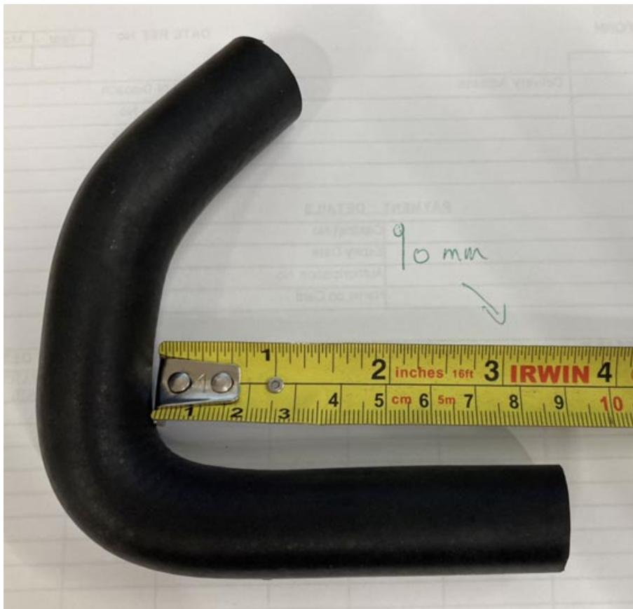
**14. Cooling hoses:** With the above removed, fit the hose assembly with the bottom hose extension. The end that fits onto the water pump housing requires a notch cut out to fit around the casting material on the water pump housing; this helps with clearance from the turbo to the intercooler pipe. See pictures right and on p. 19.
