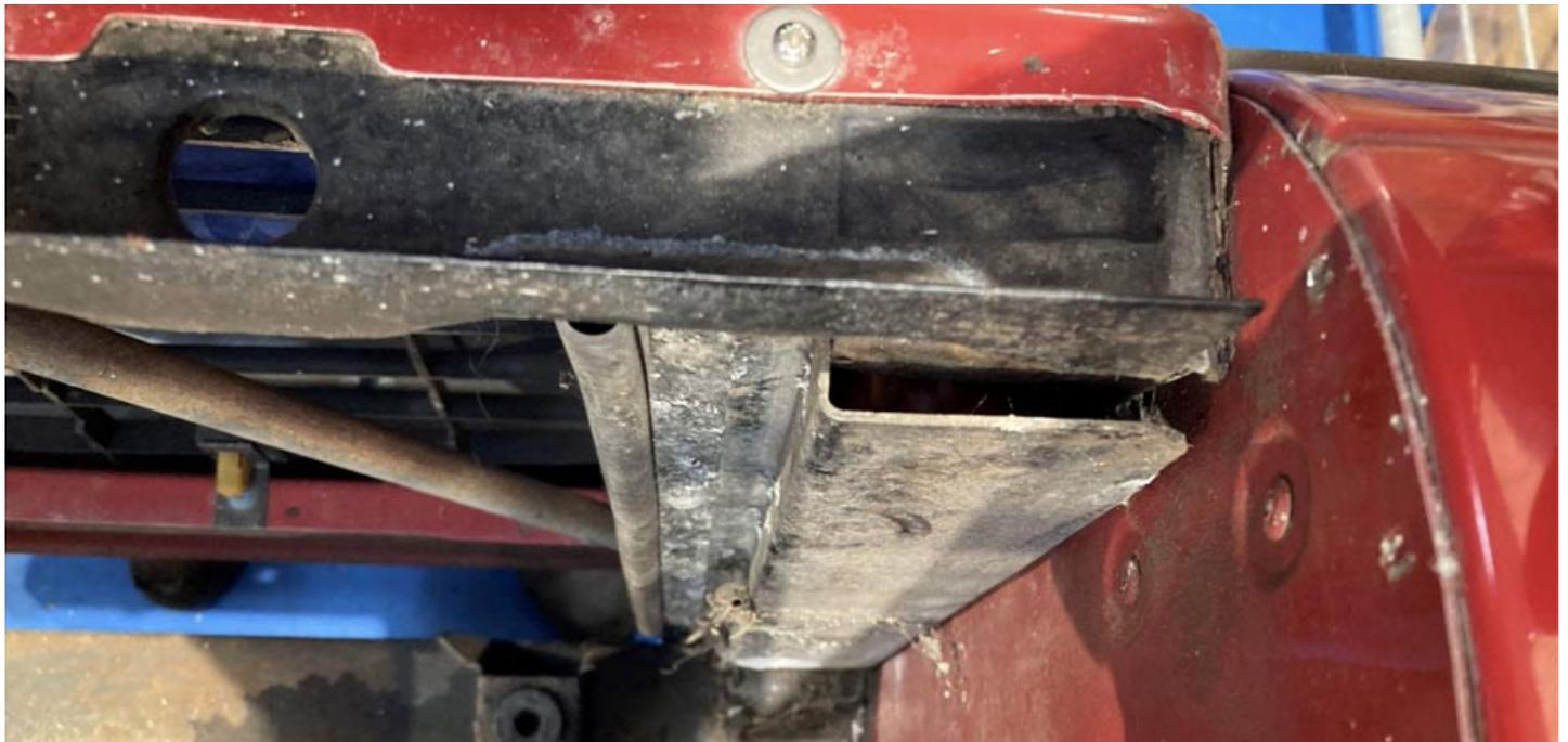
8. **Gearbox chassis brackets:** The gearbox and transfer box need to sit as far forward as possible; this is to help clearance for the new engine. Slacken the 3 x M8 bolts holding the gearbox chassis brackets to the chassis on both the LH and RH sides (6 x M8 bolts in total). With all 6 bolts loose, push the gearbox and transfer box as far forward as possible on their slots; you may need to use a bar for leverage if required. Retighten the 6 x M8 bolts. See 2 pictures below.
