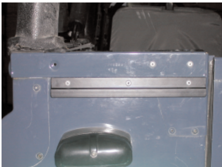
Figure 5A - rear driver's side belt rail installed with washers behind the left side 2 rivets.
