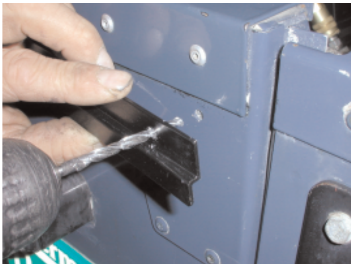
Figure 5 - use existing hole location in rear drivers side quarter panel for locating.
