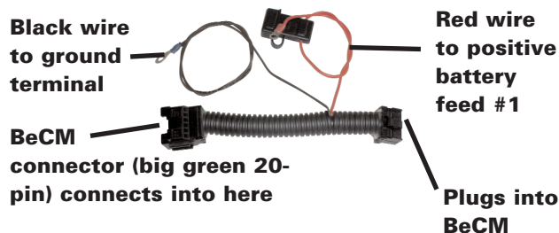
Figure 6 - EASOM Override Pigtail
