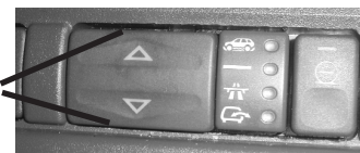
Figure 7 - Slide a thin blade type tool along the top and bottom to push the locks in while sliding the switch out.
