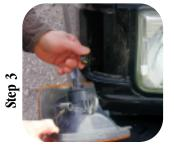
Unplug its wire connector by pressing down on the plastic lever and pulling apart.
