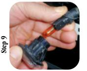
Pop out side lamp using hand pressure. Remove light bulb and replace with new amber bulb.
