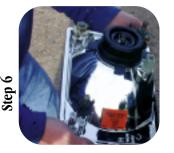
Next remove the 3 adjustable fasteners from the back of the headlamp. Take care not to rotate the fastener on the threaded stud as this will change your highlamp alignment. Simply unsnap the threaded stud from the old headlamp and snap it into the new headlamp. .
