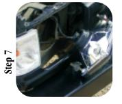
Take care to install them in the same location to avoid changing alignment. Reconnect headlamp wires and fit the headlamp to the inner panel. Then rotate the plastic fasteners to their lock position. This will securely fasten the headlamp.
