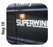
Fit new clear lamp onto bulb holder and press back into the body panel.
