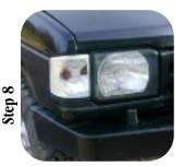
Next fit the corner lamp into position. Plug in its wire lead and pull the large wire ring into position. This will securely fasten the corner lamp.
