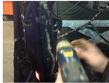
Fig 13 - Remove four rivets on regulator.
