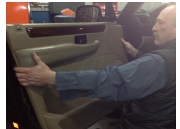
Fig 23 - Re-install door panel.
