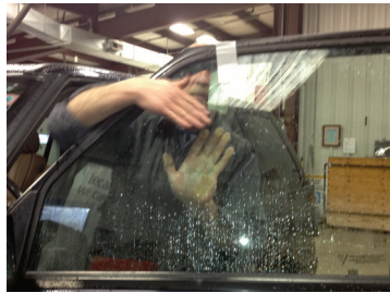
Fig 12 - Manually raise window, secure.
