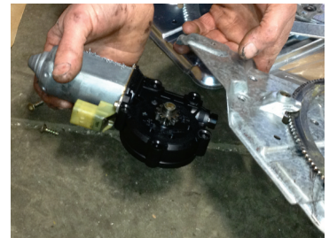
Fig 16 - Remove motor, attach to new window regulator.
