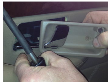
Fig 4A - Remove door latch.
