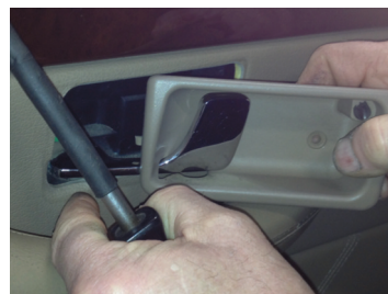
Fig 25 - Re-install door handle tray.
