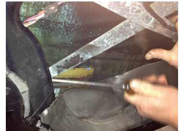
Fig 11 - Detach both ends of regulator.
