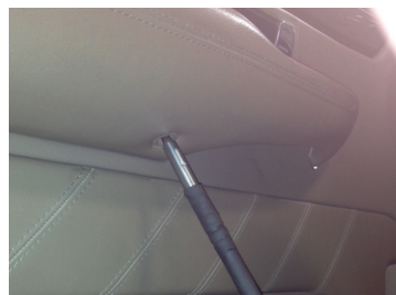
Fig 5A - Remove second door panel screw.
