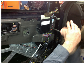
Fig 17 - Install new rivets.
