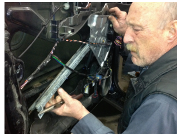
Fig 15 - Remove window regulator.
