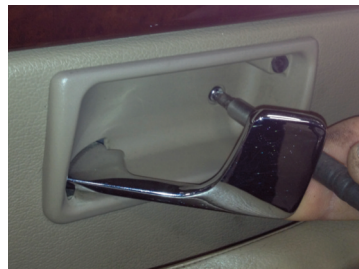
Fig 4 - Remove screw under door latch.
