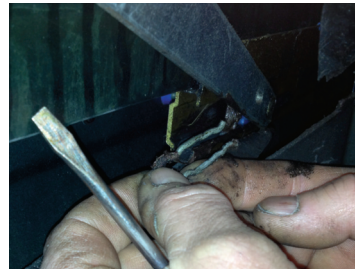
Fig 10 - Remove two clips on ball joints.
