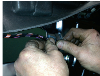
Fig 18 - Reconnect motor wiring clip.
