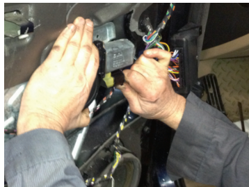
Fig 14 - Disconnect window motor clip.
