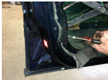
Fig 20 - Test window operation, adjust nut.
