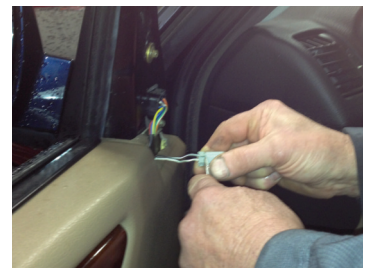
Fig 26 - Place speaker wire underneath speaker, reattach assembly.
