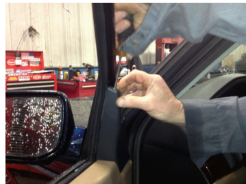
Fig 1 - Corner speaker assembly removal.
