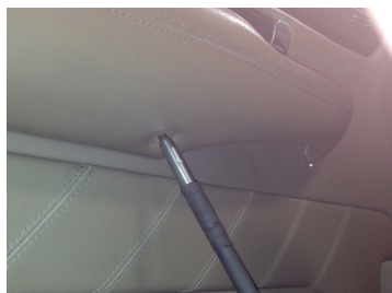
Fig 24 - Re-install door pull.
